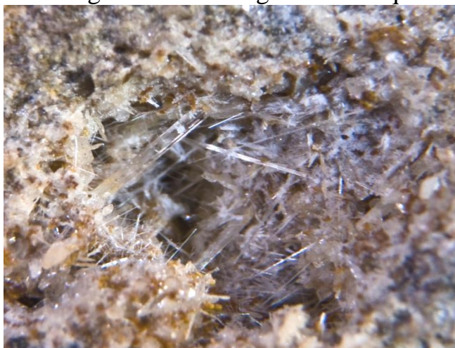
Vollastonitning mikroignasimon tuzilishi (1700 marta kattalashtirib olingan).
