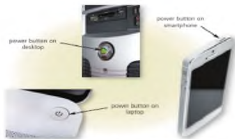
Figure 9-2 Examples of power buttons on computers and mobile devices. © Olycom / Shutterstock.com, © iStockphoto / iStockphoto.com, © iStockphoto / iStockphoto.com
