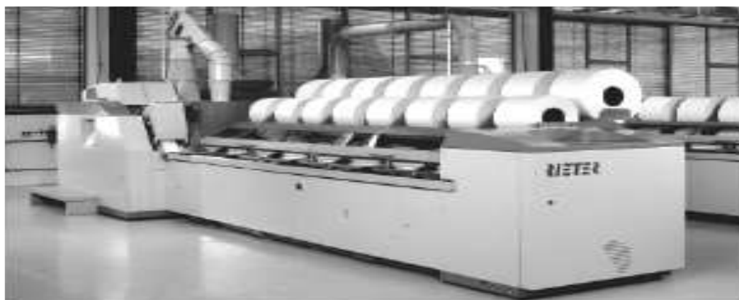
7.6-rasm. Rieter firmasining E 65 qayta tarash mashinasi
