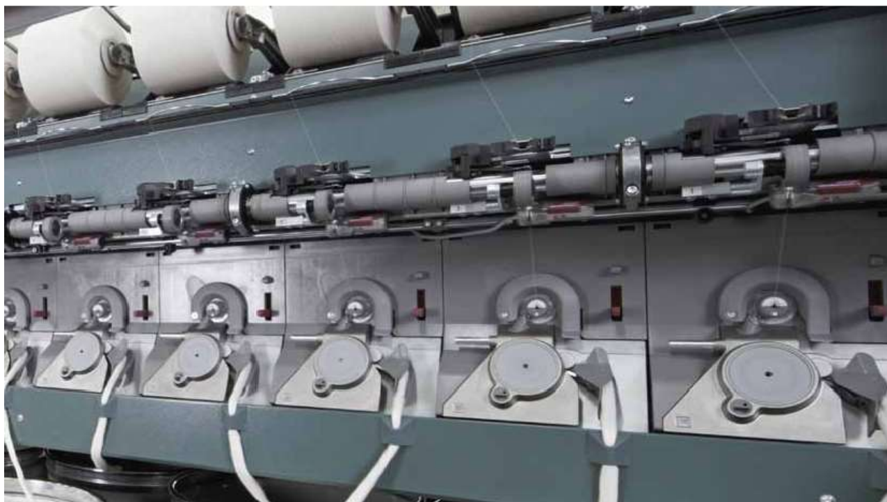
10.2-rasm. Rieter firmasining R-60 pnevmomexanik yigirish mashinasi
