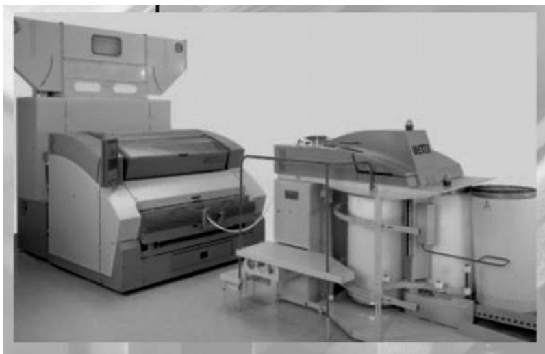
4.3-rasm. C 60 mashinasining pilta taxlash qurilmasi
