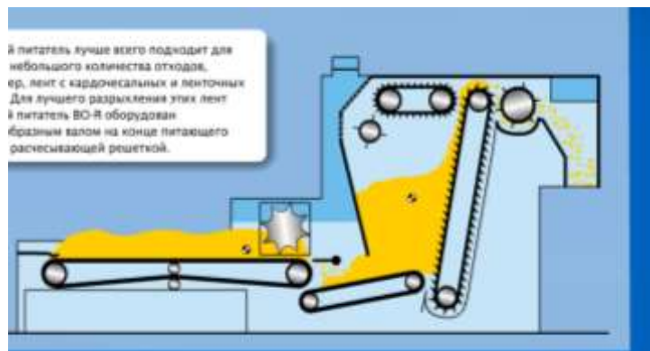
3.23-rasm Chiqindi tituvchi mashina BO-R
