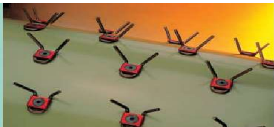
3.14-rasm UNIclen B-12 mashinasining tozalovchi baraban pichoqlari
