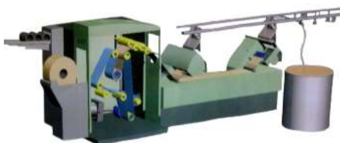
“Rieter” firmasining Omega Lap-35 piltabirlashtiruvchi mashinasi
