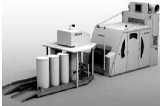
4.14-rasm. DK903 tarash mashinasi cho'zish asbobi va pilta taxlash mexanizmi
