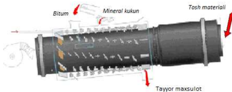
2-rasm. “DOUBLE BARREL” tipidagi quritib aralashtiruvchi baraban
