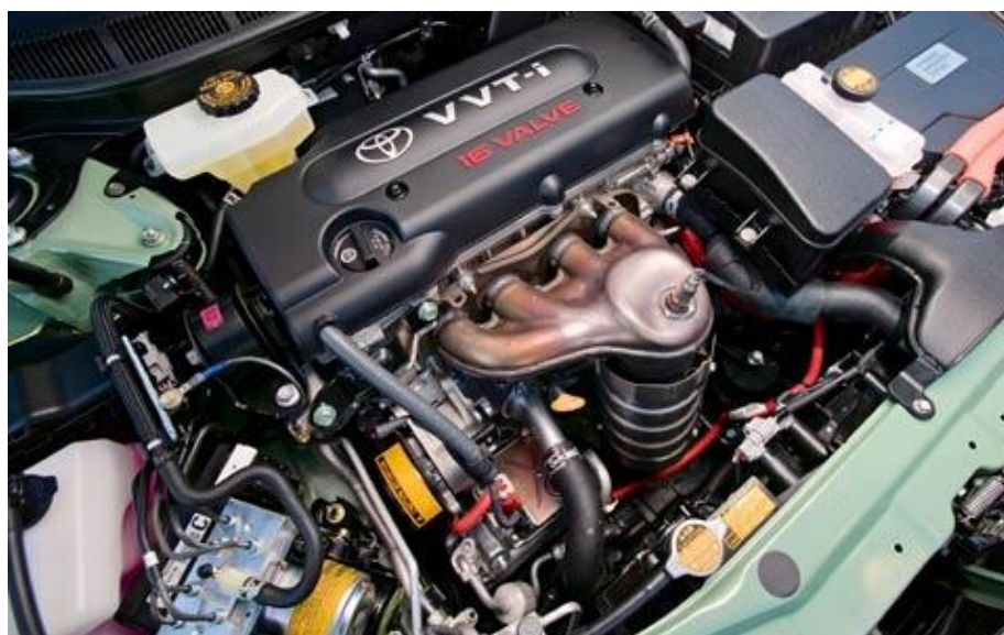
2-rasm Toyota Camre avtomobilidagi gibrid dvigatel
