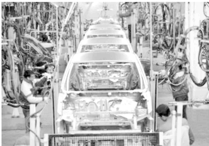
6.5-rasm. “Spark” avtomobilining kuzovini avtomatik liniyada payvandlash-yig‘ish
