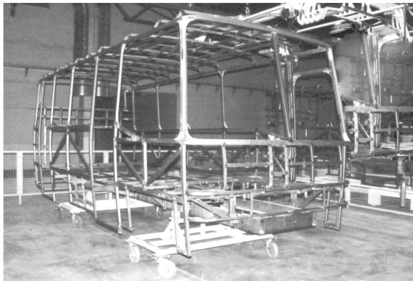
7.7-rasm. Isuzu avtobusi kuzovining ramaga yig'ilgan karkasi
