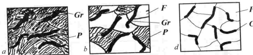
2.4-rasm. Kulrang cho‘yanning tuzilmasi tashkil etuvchilari: a – perlit-grafit; b – perlit-ferrit-grafit; d - ferrit-grafit.
