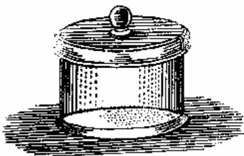
24-rasm. Quritish uchun stakancha.
