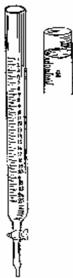
17-rasm. Titerlash uchun byuretkalar.
