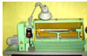
1-c rasm. yog’ochga ishlov berish “CTD-120m” tokarlik stanogi.
