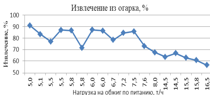
Fig. 9. The results of the industrial application of bio-oxidation product by calcination
